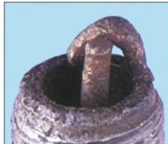
外力破坏 MECHANICAL DAMAGE
