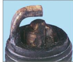
绝缘体破损 DETONATION
