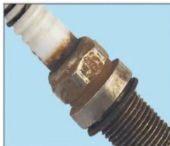
安装力矩过小 INSTALLATION TORQUE TOO SMALL
