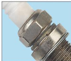
安装力矩过大 INSTALLATION TORQUE TOO LARGE
